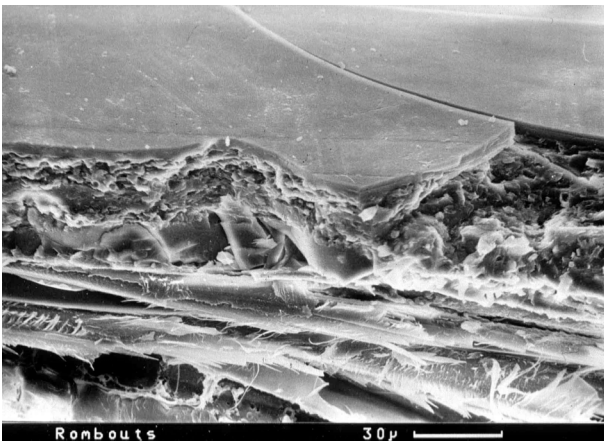
Figure 1a. Scanning electron micrograph showing wood, ground layer and varnish on a specimen by Rombouts. The scale bar in the bottom right-hand corner gives the length scale: it corresponds to 30\mu\text{m} , 0.03mm. The curving line at top centre is a crack in the surface of the varnish.
