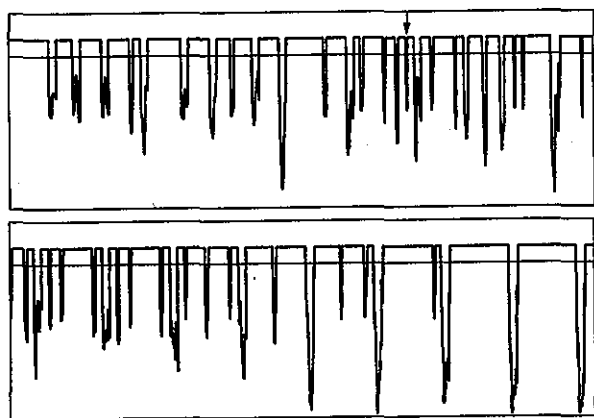
FIG. 5. The first 2400 time-samples of the string-surface velocity for a transient solution of the delta/Cremer model. The two boxes show sequential segments: the upper box shows samples 1-1200, the lower box samples 1201-2400. The horizontal segments of waveform correspond to sticking, at the bow speed v_b . The bow force had the constant value 5.5 throughout, and v_{mid}=0.7 (units and other details are described in the Appendix).
